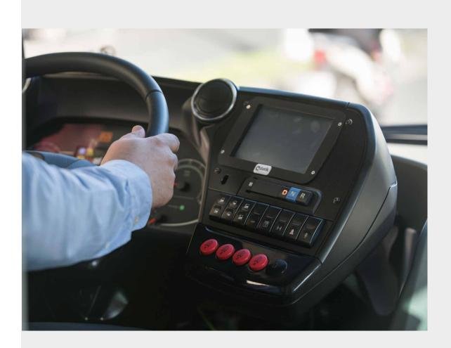
The driving position has been designed prioritizing concepts of ergonomics, comfort, functionality, safety, and service while complying with the EBSF standards (European bus system for the future–project managed by UITP and VDV).
